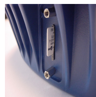
Figure 14: SIM Ready for Removal
