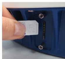
Figure 12: SIM Being Installed
