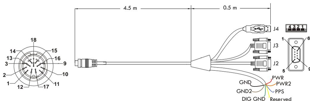
**Table 32: USB Multi-Cable Connector Pin-Outs**
