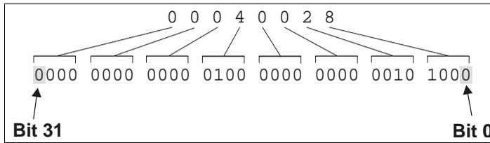
**Figure 33: Reading the Bits in the Receiver Status Word**
