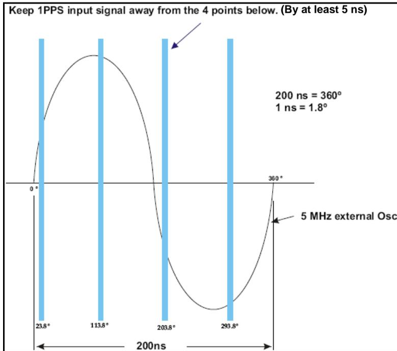
Figure 19: OEMV-3 and ProPak-V3 T Sync 5 MHz and 1PPS
