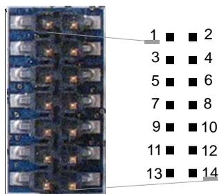
**Figure 54: Top-view of 14-Pin CAN Connector on the OEMV-3**
