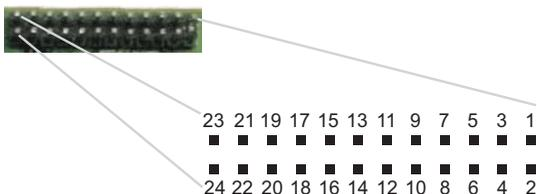
Figure 50: Top-view of 24-Pin Connector on the OEMV-2
