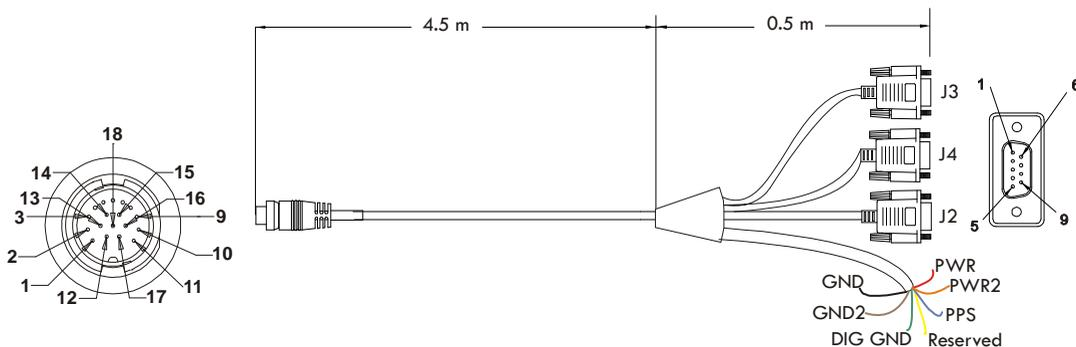
**Table 33: CAN Multi-Cable Connector Pin-Outs**
