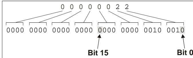
**Figure 35: Reading the Bits in the Receiver Error Word**
