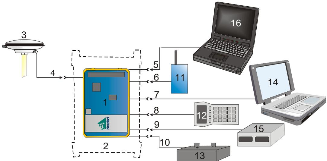
**Figure 17: Available OEM Card Connection Interfaces**
