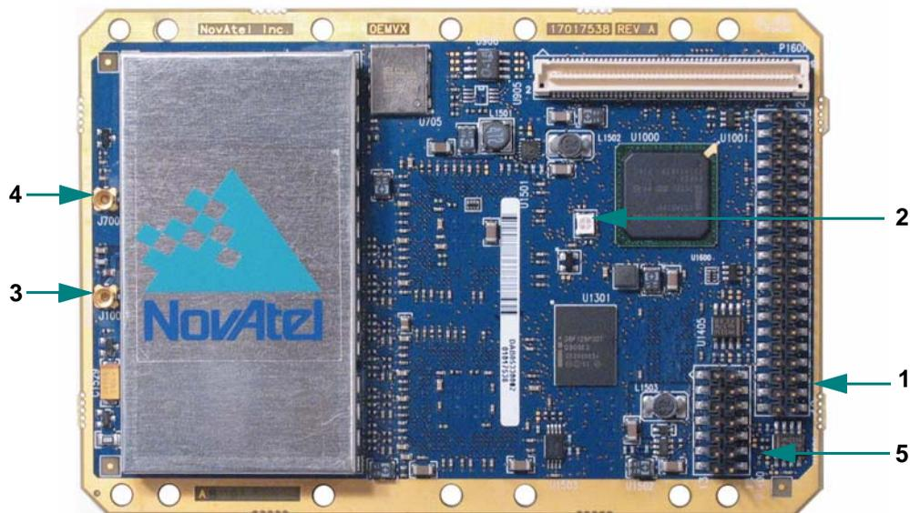
**Figure 15: OEMV-3 Connector and Indicator Locations**
