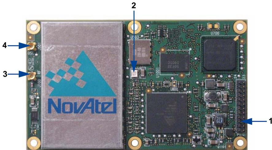
**Figure 14: OEMV-2 Connector and Indicator Locations**
