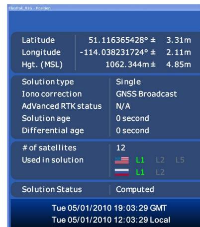
show details of the GNSS and geostationary (SBAS) satellites being tracked, select a *Tracking Status Window* (*GPS* or *GLONASS*) from the *View* menu.
