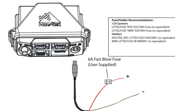
5. Plug in the adapter and/or turn on the power supply. The LED will be red when the FlexPak is properly powered.
